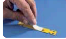
3) Seal the carrier by placing a finger on the foil and pushing forward, thus rolling over the foil and rolling off the silicon liner.
